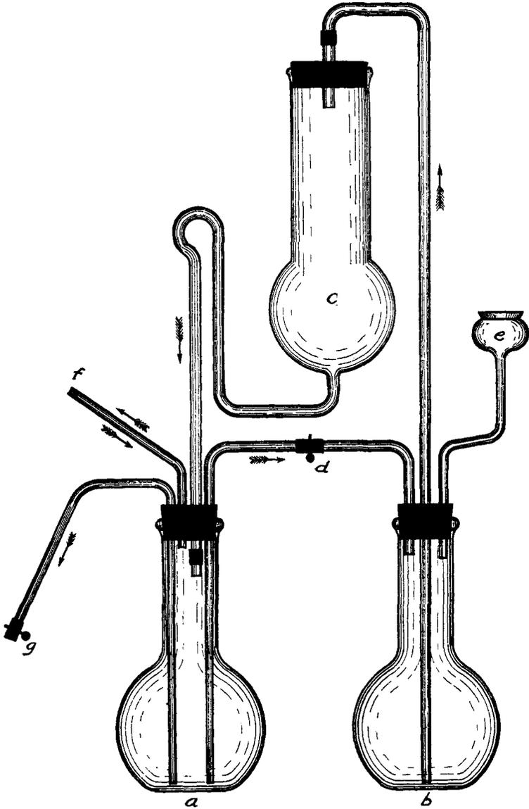
by opening *g* and blowing in at *j*. A fresh supply of water is then added, and the process continued until the extraction is completed.
